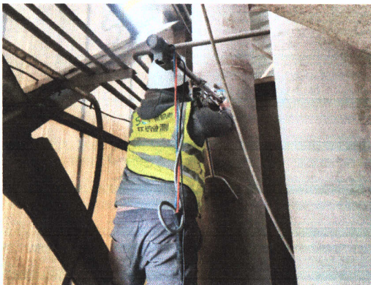
DA002 球形矿仓废气排放口采样
